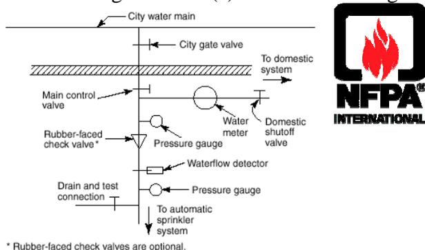
The advantage to the configuration shown in Figure A.6.2(a) is that the only shut-off valve for the fire protected system also shuts off water to the domestic system. This encourages people to keep their sprinkler systems operational.
