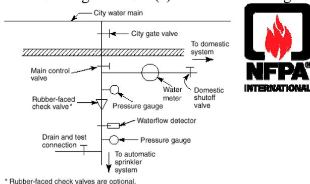
The advantage to the configuration shown in Figure A.6.2(a) is that the only shut-off valve for the fire protected system also shuts off water to the domestic system. This encourages people to keep their sprinkler systems operational.
